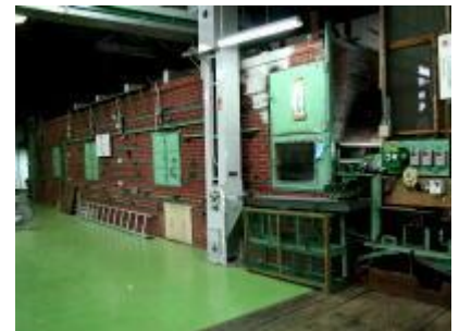
Tea leaves dry in a three or four level fire pit, heated from underneath by a burner.
